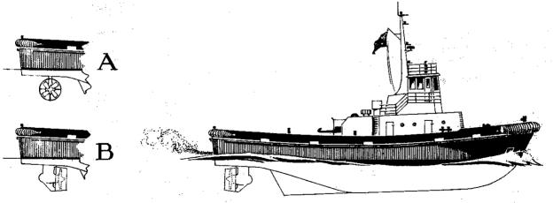
The first 'Duckpeller' tug to be built outside Japan, CAREENING COVE, was delivered by Carrington Slipways, Newcastle, to Fenwick's in mid-December. Propellers are mounted in twin units to swivel through 360° to give directional thrust for greater manoeuvring efficiency than is possible with conventional fixed screws and rudders. In the profiles above, the units are shown positioned A for lateral thrust and B for going astern. A sister vessel, SHELL COVE, should follow this January
