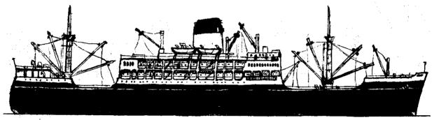
The upper illustration shows how ATHENIC and CORINTHIC appeared after being converted to purely cargo carriers. Their superstructures were originally very similar to those of CERAMIC and GOTHIC (lower drawing) the principal differences being in the funnels and the ventilators around the funnels. The last pair also had a differently shaped bow.
